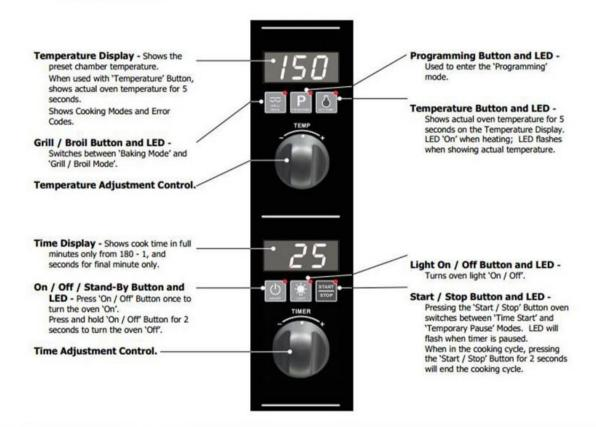
Gastronome Turbo Fan Oven Using the Oven—Manual Mode
